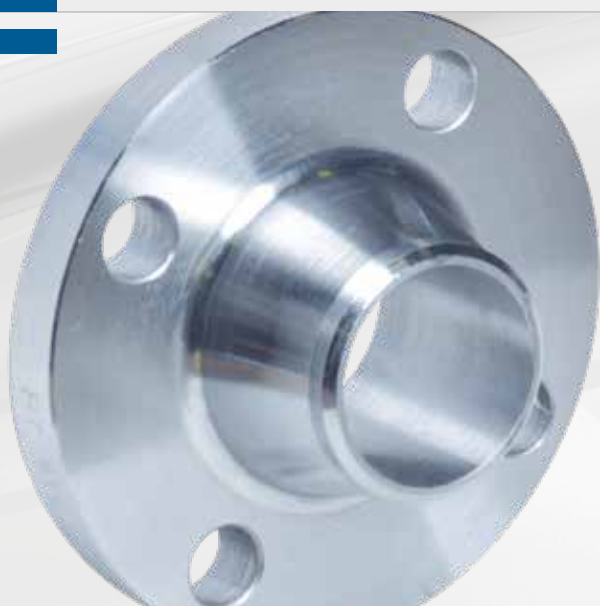
Flangia welding neck ASME B16.5 ANSI 600 lb - SCH. XS Acciaio al carbonio W.N. flange ANSI 600 lb SCH. XS - Carbon steel
