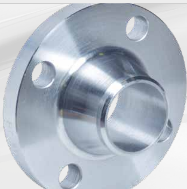
Flangia welding neck ASME B16.5 ANSI 900 lb - SCH. XXS RF Acciaio al carbonio W.N. flange ANSI 900 lb SCH. XXS RF - Carbon steel
