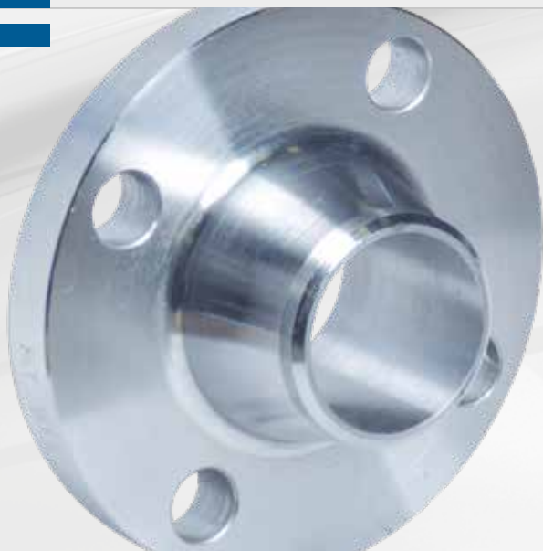
Flangia welding neck ASME B16.5 ANSI 150 lb - SCH. STD Acciaio al carbonio W.N. flange ANSI 150 lb SCH. STD - Carbon steel
